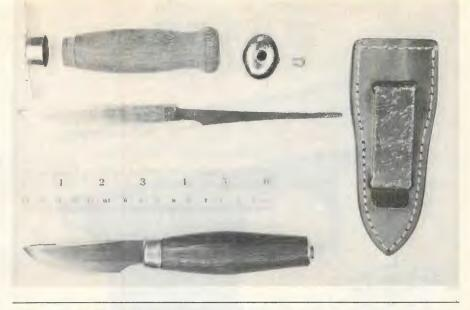
Above: The modified Mora knife described in the last letter, showing original parts above; the finished boot knife below.
